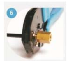
assemble the hose by positioning manual pliers on the sleeve covering its whole surface
