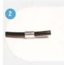
to insert the sleeve with the groove on the hose
