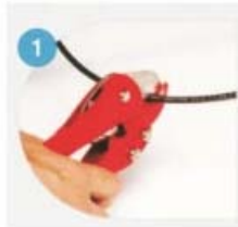
To cut the thermoplastic capillary hose
